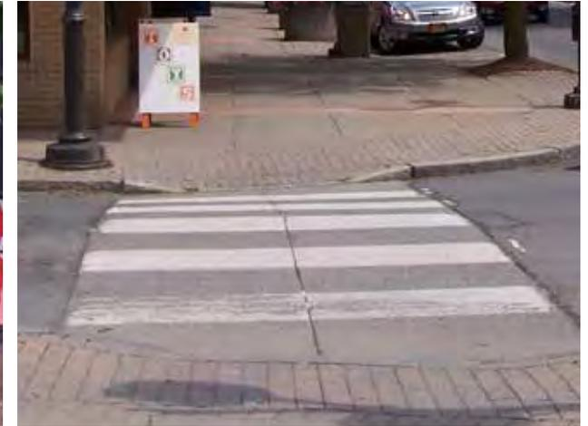
Crossing distance is shortened by curb bump-outs. Crosswalk locations are noted by curb ramps and are marked with a ladder pattern, painted the width of the crossing. Paint has faded and should be restored. Curb ramps should be upgraded to meet current ADA standards with tactile warning surfaces. Additional standard features should be considered in coordination with the NYSDOT regional office.
