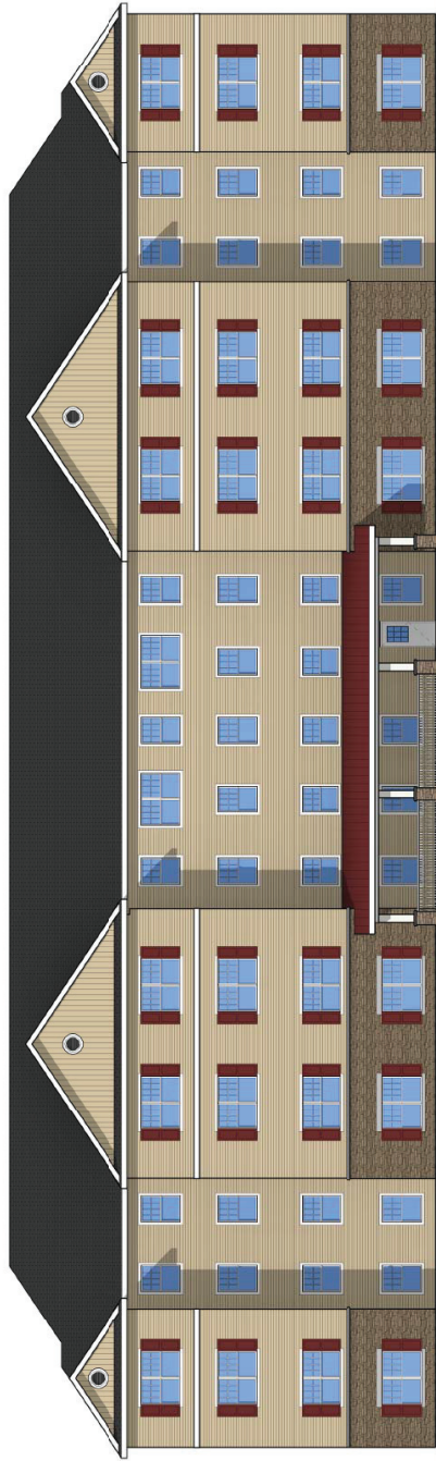
2 BUILDING A BACK ELEVATION 1/8" = 1'-0"
