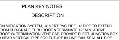
PASSIVE RADON MITIGATION SYSTEM, 4" VERT PVC PIPE. 4" PIPE TO EXTEND VERTICALLY FROM SUB-GRADE THRU ROOF & TERMINATE 12" MIN. ABOVE SURFACE OF ROOF W/ TERMINATION VENT CAP. PROVIDE ELECT. JUNCTION BOX IN ATTIC AREA NEAR VERTICAL PIPE FOR FUTURE IN-LINE FAN. SEAL ALL PIPE CONNECTIONS (TYP.)TO PROVIDE AIR-TIGHT SEAL.
