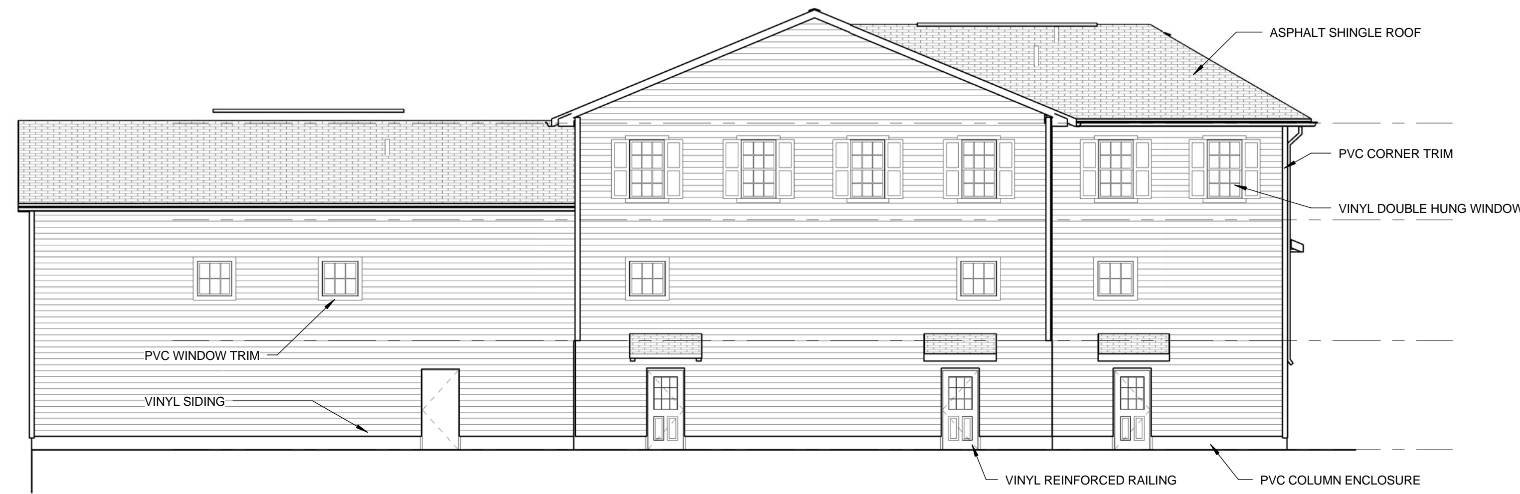
3 EXTERIOR ELEVATION - SOUTH 1/8" = 1'-0"
